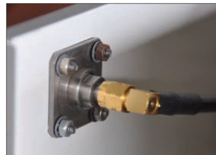
Fig. 4: The chassis-mounted antenna N-Type to SMA adaptor socket used by Colin G6MXL. Note the SMA connector which prevents any r.f. leaving the socket inside the case.
