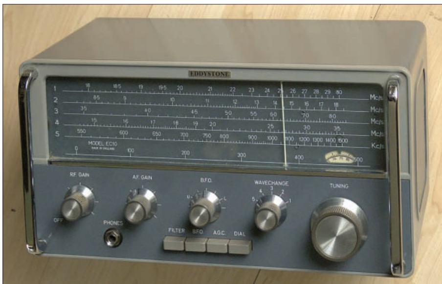
Fig. 2: The EC-10 receiver, nice big tuning scale.
