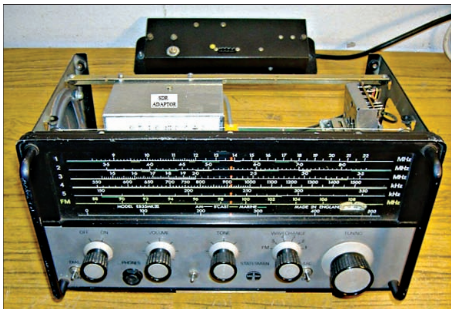
The Eddystone EB35 MkII with the SDR addition mounted in its screened box attached to the top strut at the rear of the receiver.
