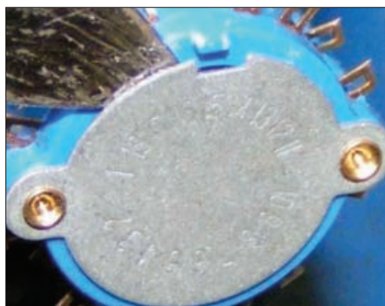
Fig. 1: Easing away the back-plate of a sealed switch, allows switch-cleaner to be squirted in.
