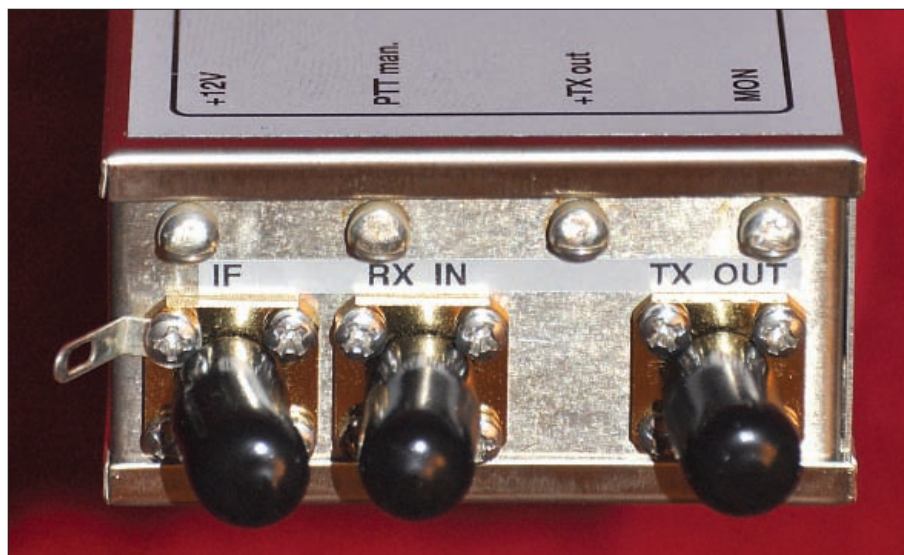
Fig. 3: The SMA connectors on the Kuhne 3.4GHz transverter are protected with black plastic covers during transit.
