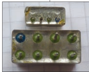
Fig. 2: Looking at the pins of the two commercial types of balance diode ring mixers
