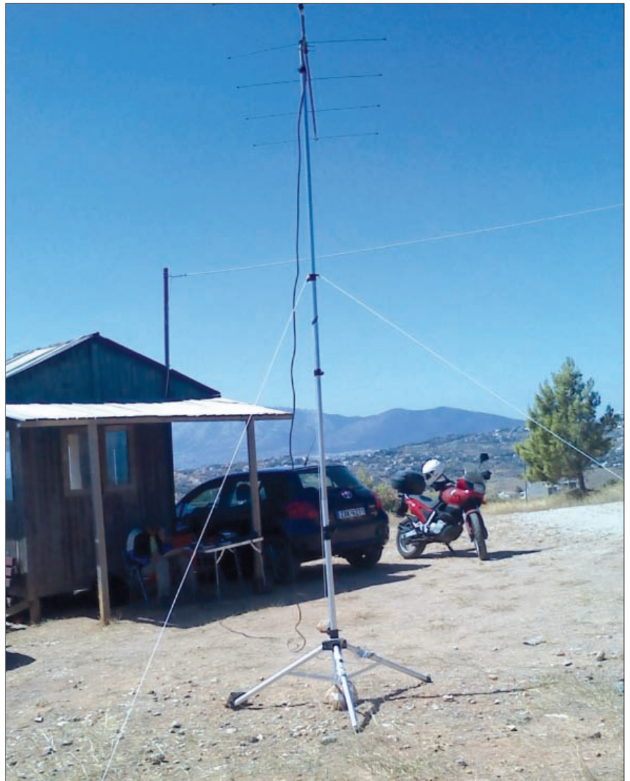
Fig. 1: Panos Dadis SV1GRN operated at the fire observatory of Pikermi, where with a Yagi antenna supported on a lightweight guyed temporary vertical mast. What glorious weather for a day out!
